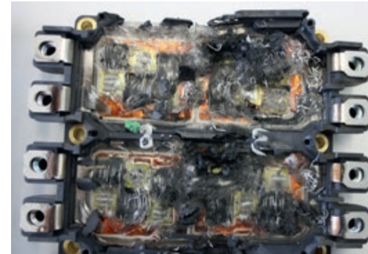
Damaged converter module
